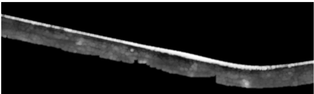
Figure 2.7: Thermal infrared image after applying blur with a circle of five pixels radius and applying dilation again with a circle of five pixel radius
