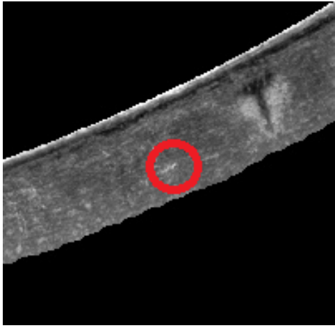
(a) Blob classified as a leak, while not corresponding to an observed leak (centre of the picture, not to be mistaken with the blob more to the upper right).
